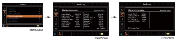
• The machine status such as the engine rpm, oil temperature, voltage and pressure etc. can be checked by this menu.
